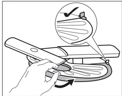
7. Reassemble the filters (B) and (C).
