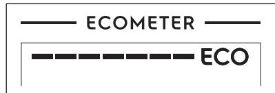
The ECOMETER indicates how the programme selection impacts energy and water consumption. The more bars are on, the lower the consumption is.
