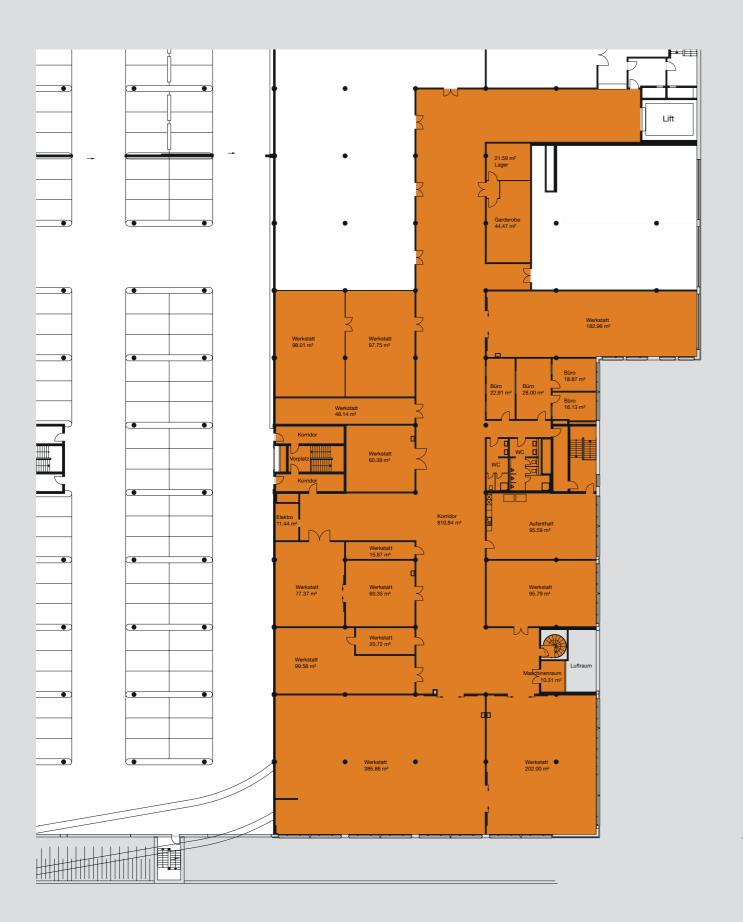
Level 5 offers a workshop area of 2'667.4 m<sup>2</sup> with two fully equipped paint booths, a fitted carpentry workshop, WC's, showers, a break room and offices.
