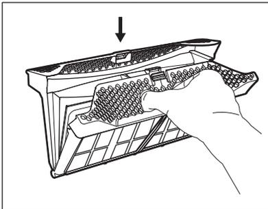
3. Use a moist hand to clean both parts of the filter.
