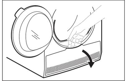
3. Turn the lever to unlock the condenser lid.
