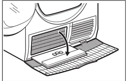
5. If necessary, remove the fluff from the condenser and its compartment. You can use a wet cloth and/or a vacuum cleaner with a brush attachment.
