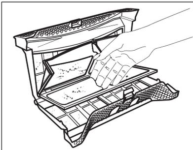
4. If necessary, clean the filter with a vacuum cleaner. Close the filter.
