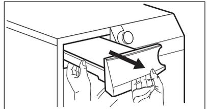
2. Pull the plastic connection out and drain the water into a basin or equivalent receptacle.
