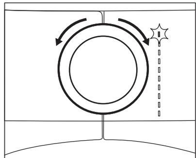
Use the program dial to set the program. The possible time to complete the program comes into the view on the display.
